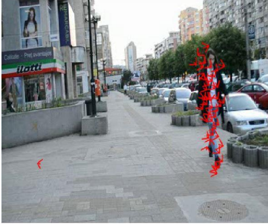
Figure 4. Sample of optical flow vectors assigned to obstacles – with red arrows
